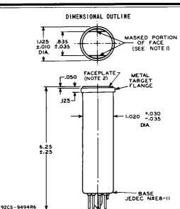
DIMENSIONS IN INCHES Note 1: Straight sides of masked portions are parallel to the plane passing through tube axis and short pin. Note 2: Faceplate glass is Corning No.7056 having a thickness of 0.094  $\pm$  0.012 inch.
